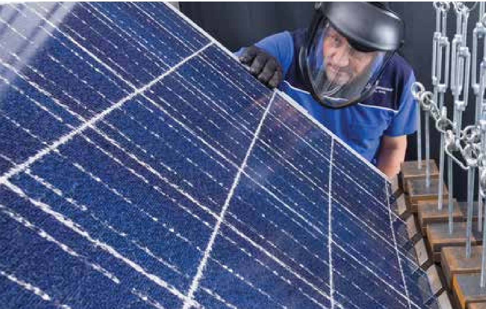
PV load testing simulates heavy snow which can accumulate on a sloping roof (Photo: TÜV Rheinland)
