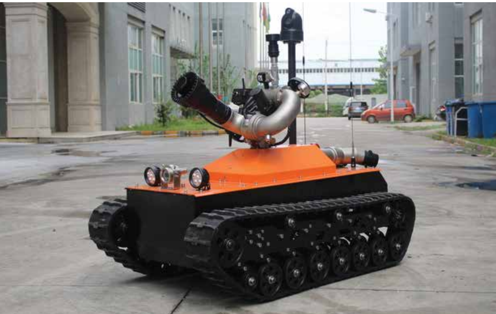
This quick-deployment RXR-M80D-1 fire extinguishing robot can be used in disaster areas such as chemical plants, subway tunnels, gas leakage, and so forth (Photo: Beijing Topsy Century Holding Co. Ltd)
