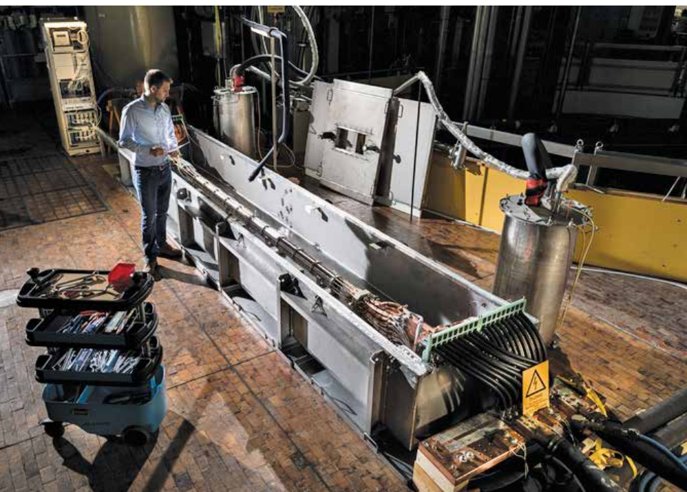
Testing superconducting cables at the Karlsruhe Institute of Technology (Photo: KIT)
